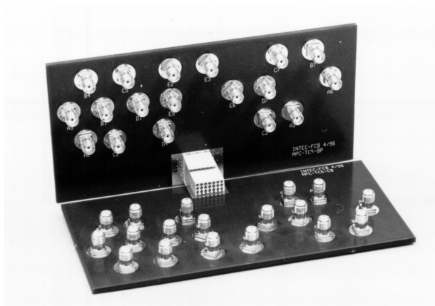
Figure 3: Test fixture for characterisation of a non-shielded backplane connector.
